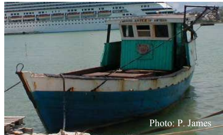
Figure 8. Traditional wooden launch with winch and trap hauler.
